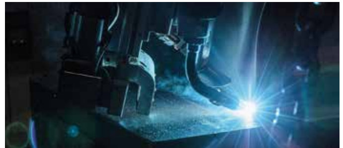
Fig. 1 The Laser Hybrid process joins aluminum and steel parts at high speeds
