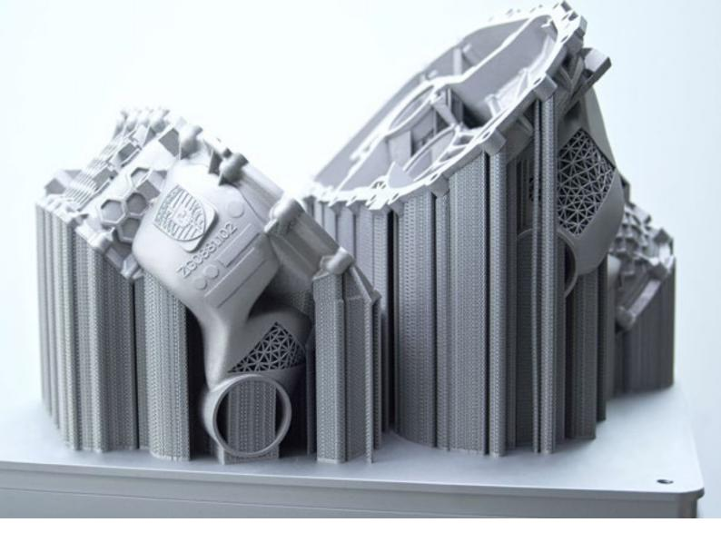
"This new manufacturing technology is technically and economically interesting for us. Possible use cases are especially prototypes in the development phase, special and small series production as well as for motor sport and classic spare parts." The E-drive unit measures 590 x 560 x 367 mm and was built in only 21 hours on the NXG XII 600.
