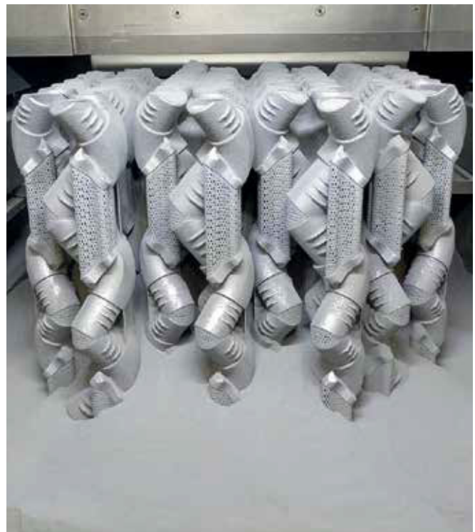
Fig. 5: 120 stacked, nested connectors printed in one process on the SLM@280 by Finnish service bureau 3Dstep Oy.
